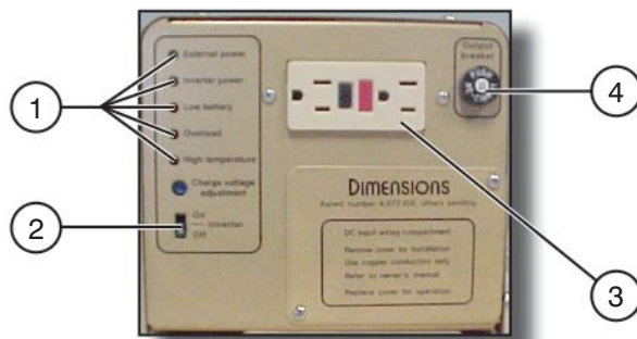
Figure 3-9. 1500W AC Inverter
