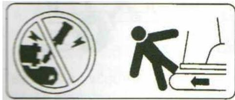
Be sure that the dozer is on the "left" side. (The dozer must be -2 sided.) If the swing frame has been turned 180°, i.e. the dozer is, seen from the operator, "behind", then the travel direction is opposite to the drive direction of the levers (when activating the drive lever forwards, the excavator, seen from the operator, will move backwards).
